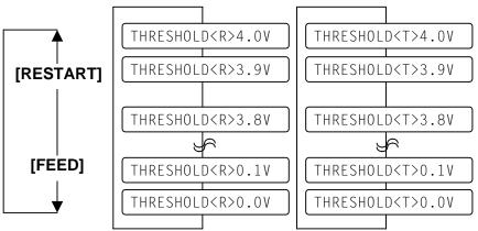
**[FEED]** key: Pressing the **[FEED]** key one time causes a -0.1V change, up to 0.0V.
